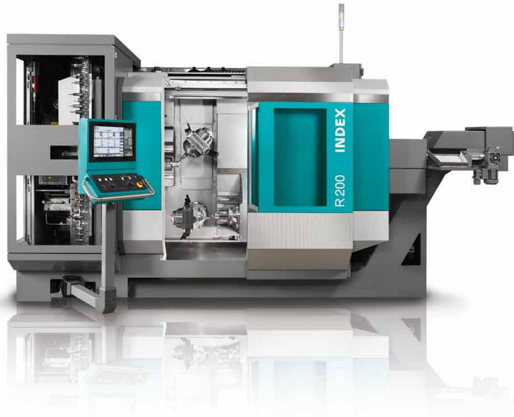
**Two milling spindles are used simultaneously and independently**
