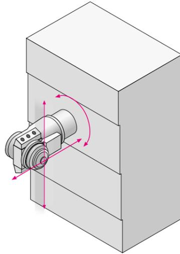
During development of the R series, emphasis was placed on achieving a high degree of stiffness, thermal and dynamic stability, and vibration damping. For this reason, a vertical cast machine bed with a heavily ribbed, enclosed modular design was chosen. The motorized milling spindles are placed in the center of the machine and are operated freely and wearfree in the Y- and B-axes via hydrostatic circular guides. The guide system contributes considerably to the
