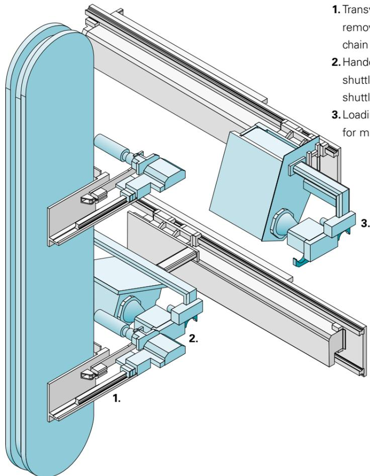
1. Transverse shuttle for removal of tools from chain magazine
